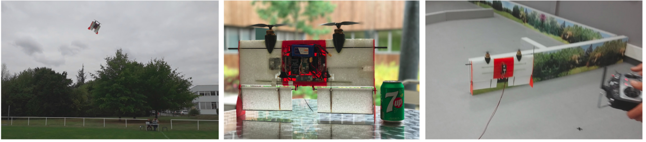
Fig. 1. The MAVION version employed throughout this work at outdoor flight (left), rest (center) and indoor flight in tail-sitting mode (right).
