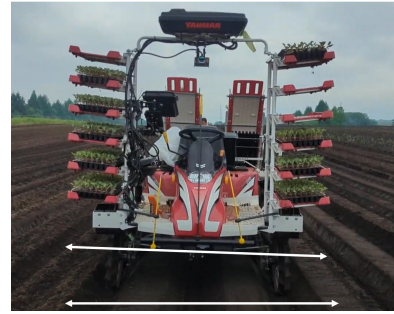
Fig. 4. Transplanter often tilts in the roll direction relative to the ridge surface depending on the groove environment.
