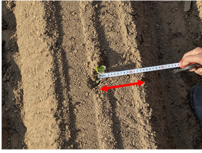
Fig. 12. Measurement of the error of transplanting on the ridge. Red two-way Arrow shows an example of left ridge.
