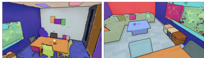
Fig. 9: Our methods do not perform well in cases where the scan sequence contains only images of the different sides of an object (chair) or surface (floor) from differing directions without any smooth transitions in between, which occurs for office2 from Replica (vMap split [20]).
