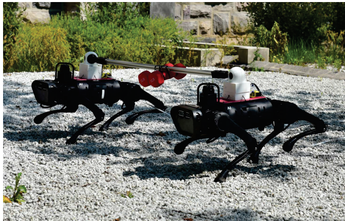
Fig. 1. Snapshot illustrating holonomically constrained quadrupedal robots locomoting on gravel while carrying a payload of 4.53 (kg).
