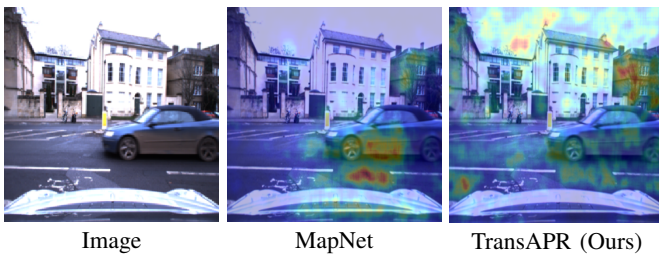
Fig. 5: An example scene selected from Oxford RobotCar and its corresponding activation maps. Compared with MapNet, TransAPR focuses on a wider area in the image and largely ignores the dynamic objects such as moving vehicles.
