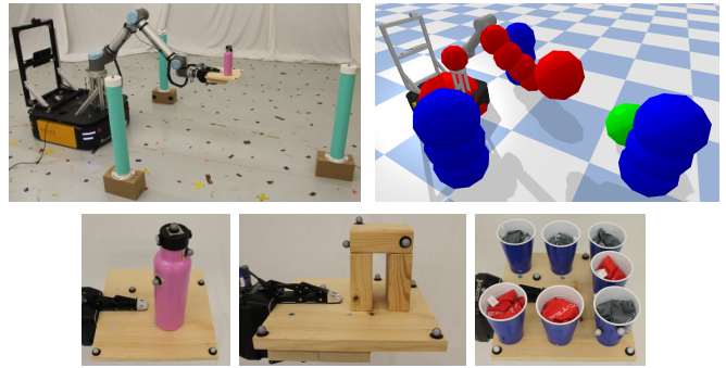
Fig. 8: Top left : Real experimental setup. Robot is shown holding the Bottle object. Obstacle locations marked with pylons. Top right : Corresponding simulated experimental setup with collision spheres on the robot in red and on the obstacles in blue. Bottom row : Bottle, Arch, and Cups object arrangements used for experiments. The arch is an example of non-coplanar contact (the three blocks composing the arch are not attached together). The bottle is filled with sugar and the cups each contain bean bags instead of liquid to avoid spills in the lab.
