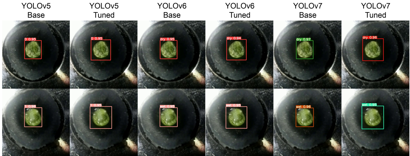
Fig. 12: Correct wetness detection results on a single orange stem by all YOLO models. Top row panels correspond to dry status while bottom row panels to wet status.
