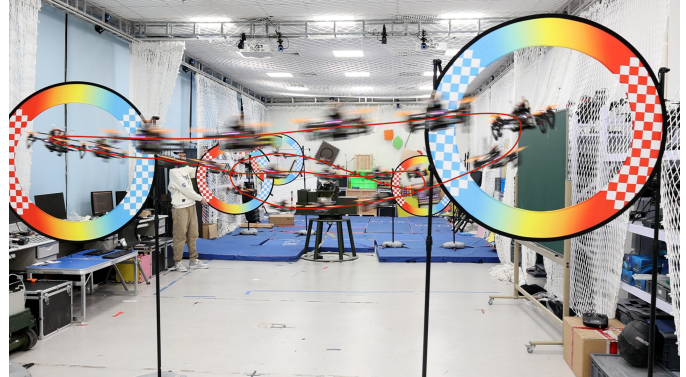
Fig. 1. Quadrotor racing through circles at a maximum speed of 10.6 m/s. The circles have a radius of 0.8 m, with four stationary circles and one moving circle held by a person. The time-optimal trajectory is quickly replanned when the position of the moving circle changes. Our proposed methods enable the quadrotor to efficiently replan and accurately track the updated trajectory in a fast and precise manner.
