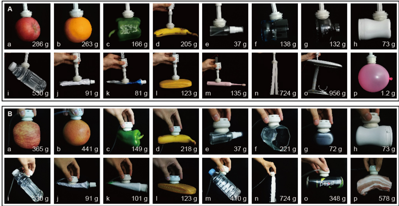
Fig. 7. Demonstration of shape-conformable suction cups picking up a variety of real-world objects. (A) Picking-up scenarios of S_{Disp} . (d), (e), (i) and (m) are with large curvature, (i), (n) and (o) are heavy, (j) and (k) are uneven, (l) has textures, (n) has corners, (k) and (p) are deformable. (B) Picking-up scenarios of S_{Force} . (d), (e), (g), (i), and (m) are with large curvature, (i), (m) and (n) are heavy, (j) and (k) are uneven, (l) has textures, (f) and (n) have corners, (k) and (p) are deformable.
