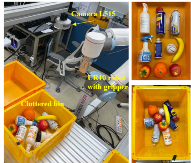
Fig. 8. Our bin picking experiment system: depth camera L515, Universal Robots UR10, Parallel OnRobot gripper, and 2 bins for picking and placing.
