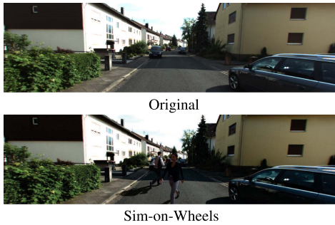
Fig. 6. Sim-on-Wheels on KITTI-360: Two jaywalkers on a street are simulated on top of KITTI-360 camera data.
