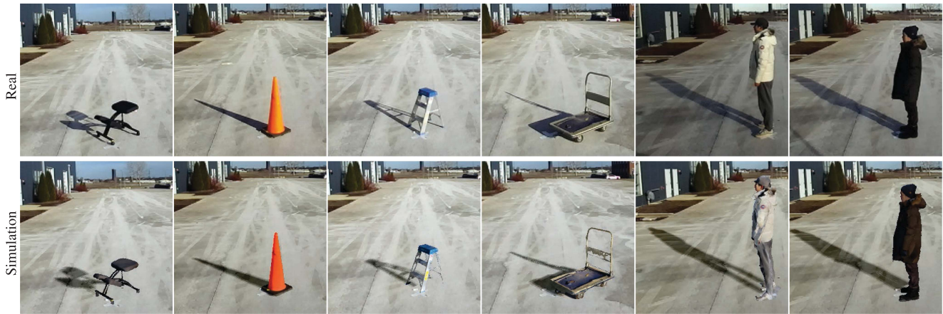
Fig. 3. Rendering Quality. We evaluate the quality of insertion rendering by comparing reconstructed 3D humans/objects in Sim-on-Wheels with their real-world counterparts under the same pose. The results demonstrate that our real-time insertion rendering can produce realistic, high-fidelity appearances, and cast-shadows. Table III quantitatively measures the sim2real gap.
