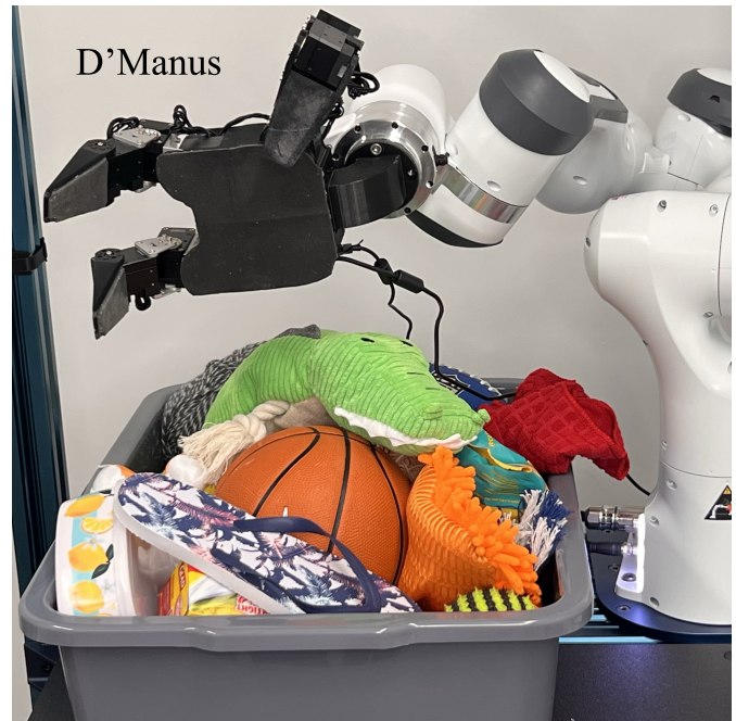
Fig. 1: The D'Manus – a low-cost, 10 DoF, reliable prehensile hand with all-over ReSkin [9] sensing.
