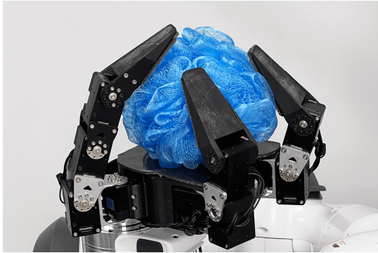
Fig. 4: Data collection setup: Tactile data is collected by placing the object on the palm and executing a human-scripted interaction policy for motor babble.
