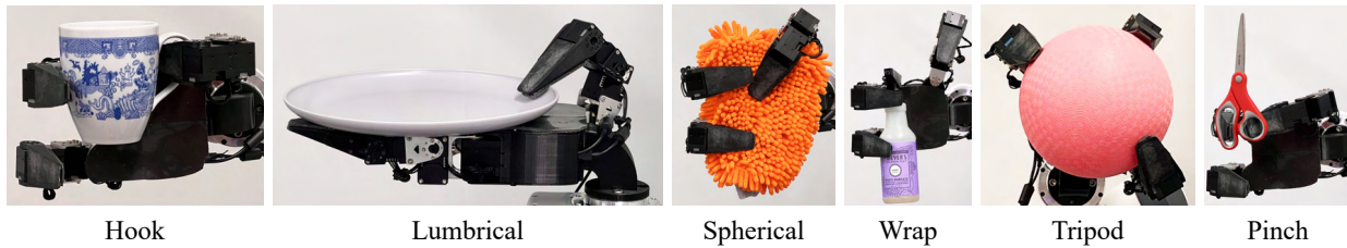
Fig. 8: Illustration of the D'Manus grasping different objects using a variety of grasps [33, 34]
