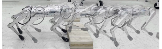
Fig. 1. Our Imitating and Finetuning Model Predictive Control (IFM) framework can learn a robust, symmetric, periodic, and efficient policy that enables the Mini-cheetah robot to overcome a 7.5cm height obstacle.
