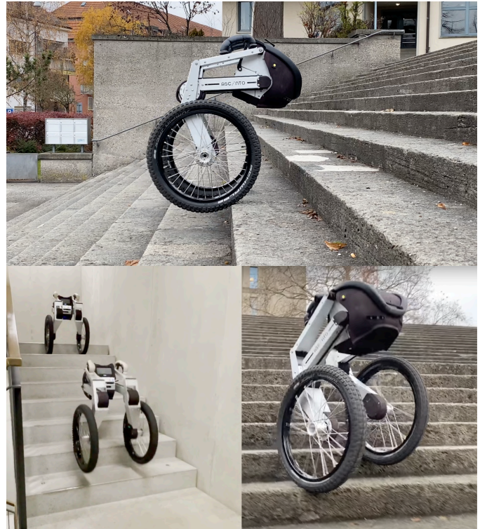
Fig. 1. Top and bottom left : The new Ascento robot climbing a stairway by repeatedly tracking motion trajectories optimized for a single step. The step height of the two stairs are 14.5 cm and 17 cm, respectively. Bottom right : Driving down a stair using only the proposed proprioceptive tracking controller. We remark that all motions shown in the video https://youtu.be/Uxt2wTI0m5o , which includes climbing the stair shown on the top, were performed using the TO scheme and/or the tracking controller proposed in this work.
