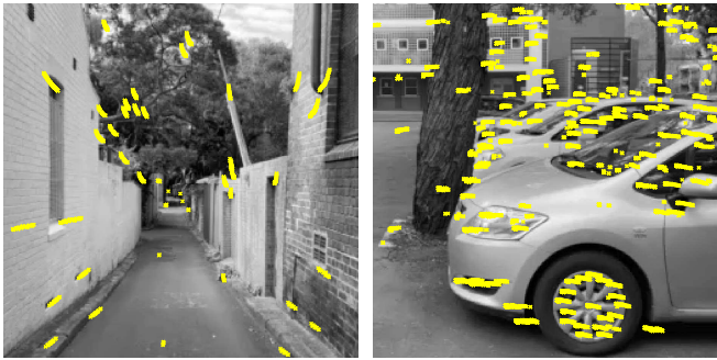
Fig. 2. (left): In 3D scenes under general 6-DOF platform motion, features in a burst exhibit apparent motion that is well approximated by line segments, even under platform rotation; (right): In the special case of a platform moving orthogonal to the principal axis of the camera, the apparent motion follows parallel line segments. We exploit these observations to search either 2D or 1D spaces of linear apparent motion to detect BuFF features.
