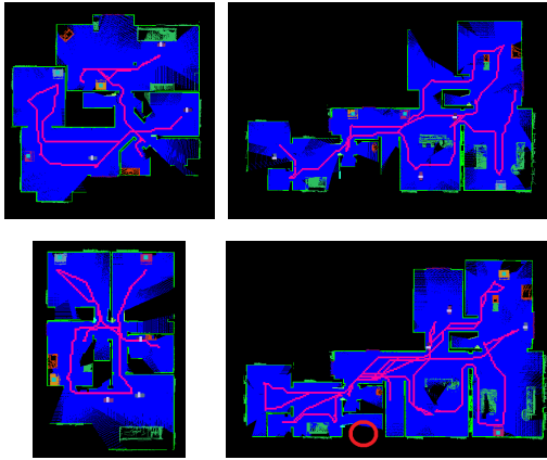
Fig. 3. Example trajectories of HIMOS in unseen apartments. Black: unexplored, blue: free space, green: walls, red: agent trace, grey: (found) target objects, other colors: miscellaneous objects. Bottom right: the agent failed to find the last object, marked by the red circle, in the given time.
