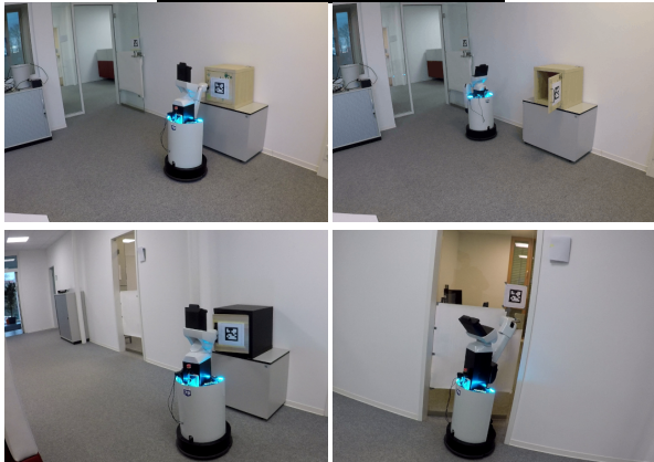
Fig. 4. Top: map of the real world environment. Initial door state and cabinet positions are randomized between episodes. Below: example trajectory in the real world. From top left to bottom right: the agent decides to look inside a target object, then navigates to the hallway, opens a different cabinet and finally opens and drives through a closed door.
