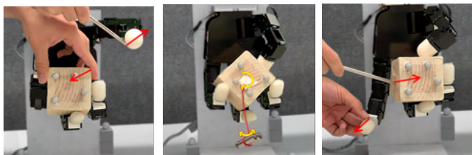
Fig. 18: Testing the robustness of our control approach by applying various perturbations to the fingers and the object during the finger-gaiting task: (left) perturbing thumb, (middle) attached pendulum that weighs as 20% of the cuboid, generates dynamic perturbations during manipulation, and (right) perturbing object and pinky finger.
