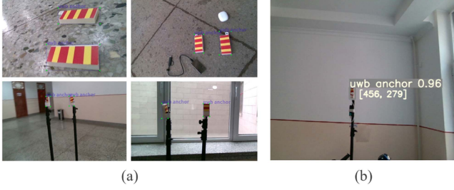
Fig. 3. (a) Labeled images for the UWB anchor dataset. (b) Detection result of UWB anchor by TPH-YOLOv5.
