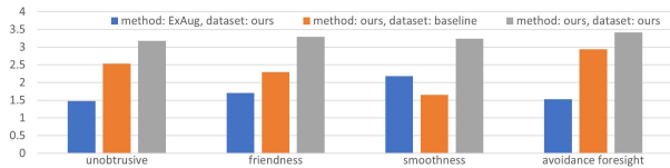
Fig. 7: Evaluation of socialness by human rating. The values are average of scores from 17 subjects. Larger is better in all ratings.
