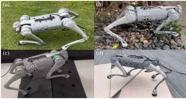
Fig. 8: The robustness test is performed where the hardware failure is triggered and the robot is commanded to locomote on various terrain roughness.
