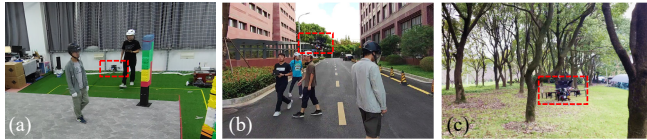
Fig. 15. The testing scenarios for obstacle avoidance. (a) and (b) are dynamic environments. (c) is a static environment. Red rectangles outline the quadrotor.
