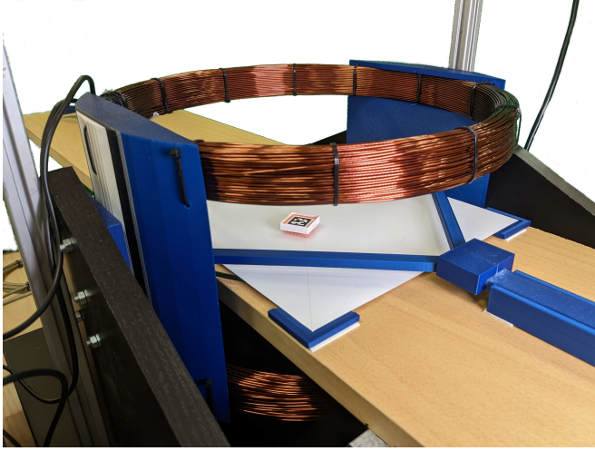
Fig. 2: Bristle-bot in Helmholtz coil, which generated a homogeneous vertical magnetic field. The upper coil ring was placed above the workspace, and the lower coil ring was placed under the workspace (only partially visible).
