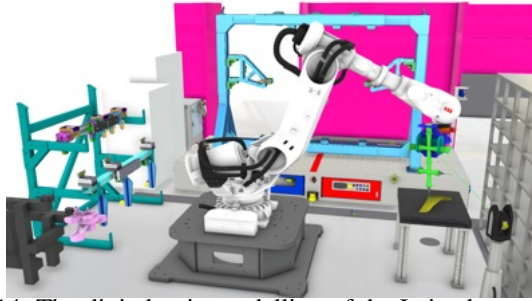
Fig. 14: The digital twin modelling of the Leica laser tracker in VC. If the laser is blocked, the line will be shown in red, otherwise it will be in green.
