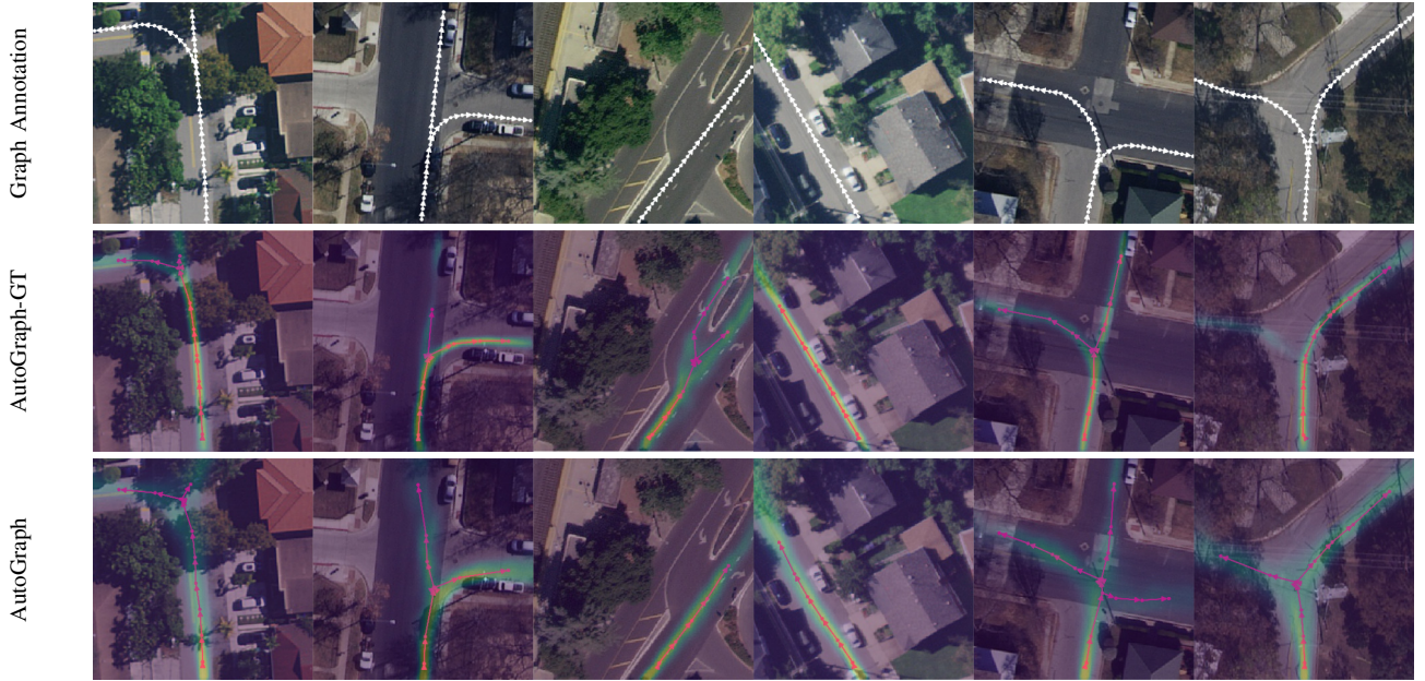
Fig. 5: Qualitative results of our models for the Successor-LGP task. We visualize the successor heatmap and the graph generated from it for our human-supervised model AutoGraph-GT and our tracklet-supervised model AutoGraph.
