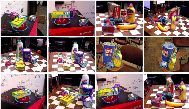
Fig. 4. The qualitative results on YCB-Video. The ground-truth poses are indicated by navy blue points, while our predictions are represented by other colors. The first two rows are correct examples. The images of the last row are the failure examples, which are mainly caused by serious occlusion.
