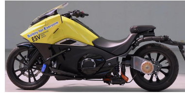
Fig. 1. Motorcycle with rear-wheel-swing assist mechanism. This experimental vehicle was developed based on a mass-produced motorcycle
