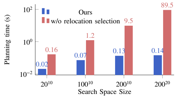
Fig. 5: Planning time (in log scale) with respect to search space size for planning robot contacts for cube sliding. We have \text{search space size} = \text{candidate contacts}^{\text{trajectory size}} .
