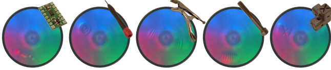
Fig. 4. Tactile images during contact of AllSight with (left to right) a circuit board, a screw driver, a locking pliers, a screw and an embossed 'x'.
