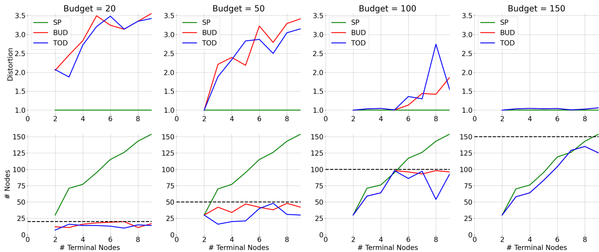
Figure 6: Comparison on distortion (top row) and number of nodes after compression (bottom row) for BUD-Lite and TOD-Lite against computing the shortest paths (SP) and pruning all nodes that are not on them. The dotted lines mark the communication budget.
