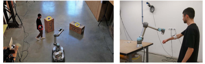
Fig. 3. Setup of the experiments with two obstacles (yellow circles) and a wrist band tracking the human operator (red circle).
