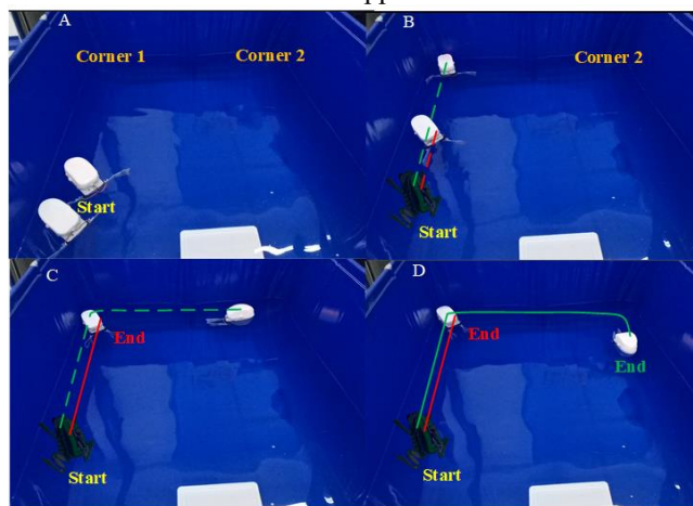
Fig. 11. Environmental adaptability experiment. The front and rear are frog-inspired swimming robots with origami and open-close flippers, respectively. Their corresponding locomotion trajectories are represented by green lines and red lines.
