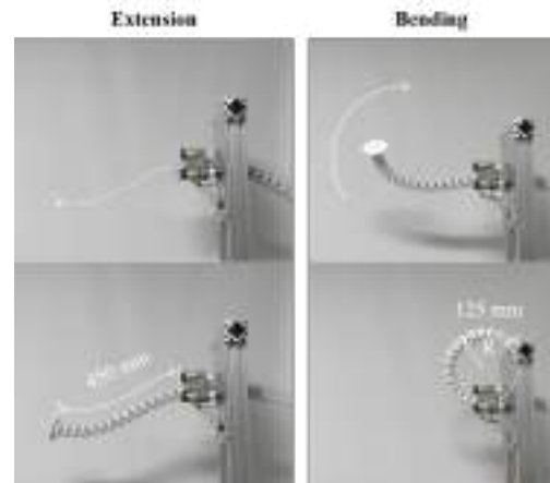
Fig. 14. Snapshot of the proposed robot during extension and bending. The robot can extend from a length of almost 0 mm up to 450 mm and can bend with a minimum bending radius of 125 mm.
