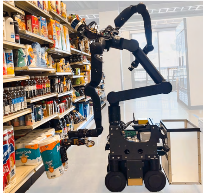
Fig. 1. Grasping bulky items from densely packed shelving with the hybrid adhesion and suction picker on TRI's TTT robot [7, 8].
