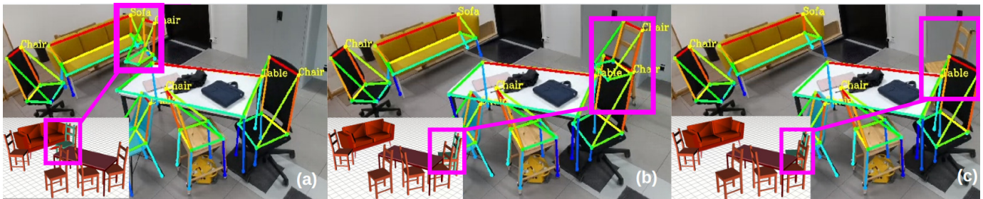
Fig. 8: Examples of predicted 2D keypoint skeletons and tracked 6D poses in presence of occlusions in a cluttered living room.
