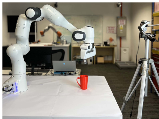
Fig. 1. Illustration of a single-camera visual policy setup for robot manipulation tasks, with a front-facing third-person camera.
