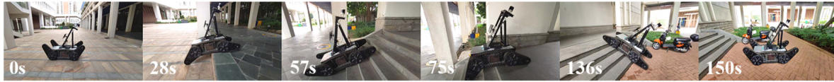
Fig. 9. Snapshot of one real-world experiment with multiple terrains, with a total distance of about 24 m. The robot needs to first pass through a platform with a height of 0.3 m (28 s), then traverse six steps (0.16 m high and 0.3 m wide) (57 s and 75 s), and climb down four steps of the same size (136 s) to reach the ground (150 s) after turning in the corridor.
