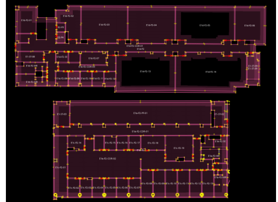
Fig. 1. Open Street Map Area Graph maps for the two experimental datasets Seq01 (top) and Seq02. We can see areas demarcated by pink polygons and passages (doors) as red lines, that are connections between areas and semantic information in terms of room names and passages. Yellow dots are polygon coordinates which form areas and passages.
