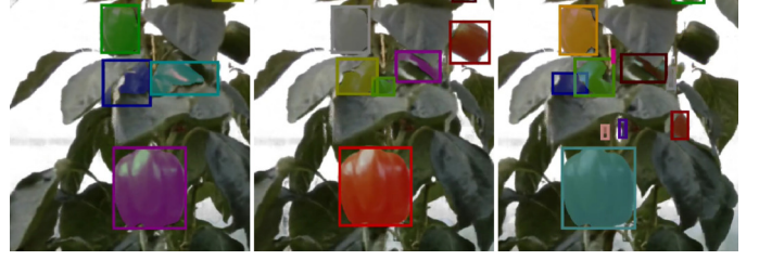
Fig. 2: Still-image panoptic detector producing inconsistent instance IDs and false positives in a sequence of frames
