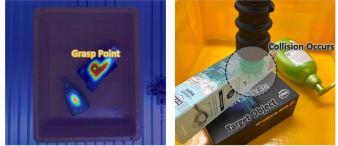
Fig. 9. Failure case of the model trained without collision evaluation. (Left) The grasp candidate has been sampled near the edge of the object. (Right) Collision occurred between the gripper and the object when grasping the target object.
