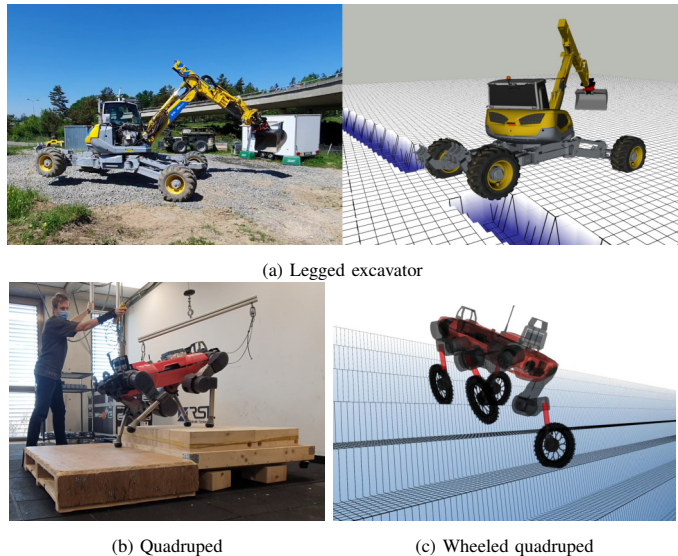
Fig. 1: a) HEAP overcomes a virtual bridge too narrow to drive over it. Hence, the stepping behavior emerges. We did not dig a ditch in our testing field. However, the map supplied to the planner contains it. Left: HEAP driving on three wheels over the bridge. Right: Visualization of the map the planner sees. b) ANYmal climbing consecutive steps. c) ANYmal on wheels stepping up the stairs (plan visualization). All the motions are also shown in the accompanying video https://youtu.be/iQiNAy6sLlo .
