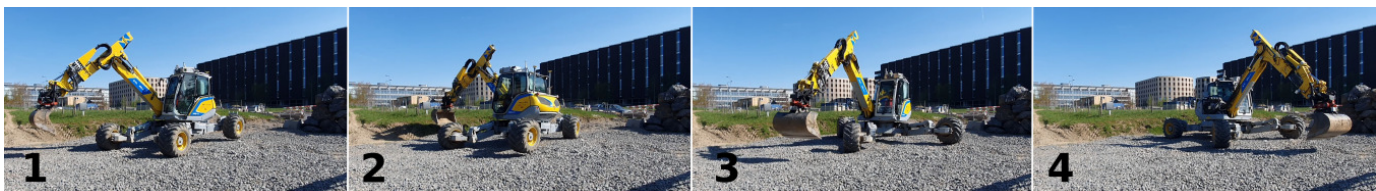
Fig. 22: HEAP performing a stepping turn in place. The x - y position stays approximately the same, while the azimuth of the chassis changes.
