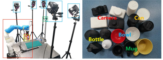
Fig. 5. (a) The data capturing system. The red, green, blue and yellow boxes indicate the Xarm robot arm with Geisight tactile sensors, the RealSense D415 RGB-D sensor, the NOKOV motion capture suite and the in-hand tracked object, respectively. (b) Object categories and instances.
