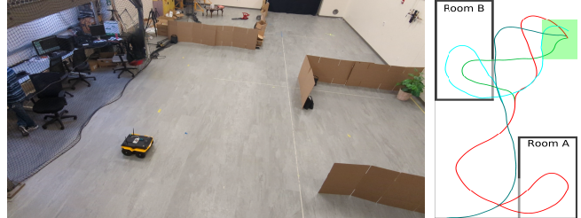
Fig. 1: Search-and-rescue scenario. Left: a robot is navigating a building with unknown room blockage and human states. Right: computed robot strategy that reacts to all possibilities of room blockages and human presence in each room. Each colored trajectory is a possible evolution of the reactive strategy.
