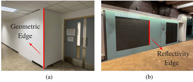
Fig. 5. Typical examples of two types of edges. (a) A geometric edge due to different reflecting angle; (b) A reflectivity edge due to material difference.
