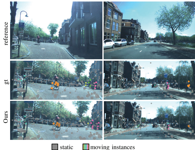
Fig. 5: Qualitative results of our Radar Instance Transformer on the validation set of View-of-Delft. The camera images are shown for reference. The ground truth (gt) instance labels and the corresponding instance predictions are projected into the reference image. The ground truth and the predictions are cropped for better visibility.
