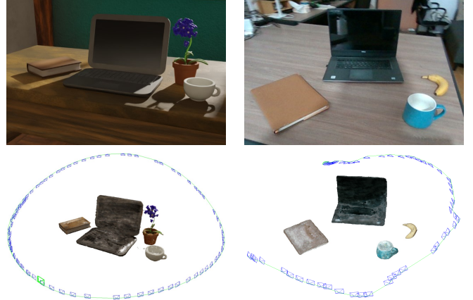
Fig. 1: RO-MAP can localize and reconstruct objects in the scene online. Each object instance is represented by a NeRF, which implicitly learns dense geometry from monocular input.
