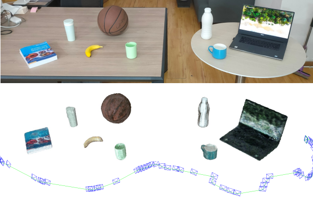
Fig. 7: (Top) The scene of the challenging real-world sequence. (Bottom) Dense object map and constrained camera motion trajectory.
