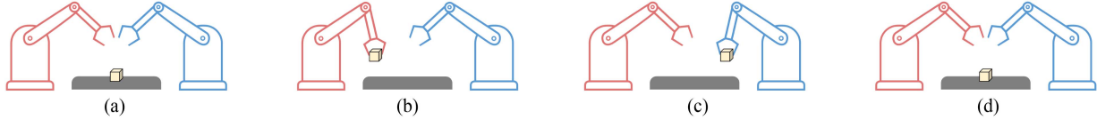
Fig. 3. (a) Figure shows the starting task space element of the system where the object is at rest at a stable pose on the table. (b) Pick action results in a switch to the middle left task space element where the red robot is grasping the object. (c) Handoff action creates another switch transferring the object from the red robot to the blue robot. (d) Finally, a place action returns the system to a stable pose task space element.
