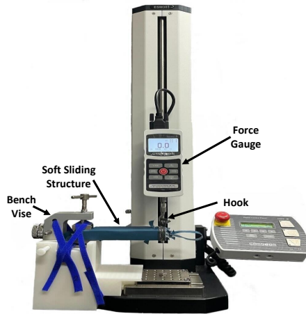
Fig. 6. Experimental setup for the bench test. The soft sliding structure is firmly clamped to a bench vise on one end, while the other end is attached to the hook of a force gauge, ensuring a stable and controlled bench test setup.
