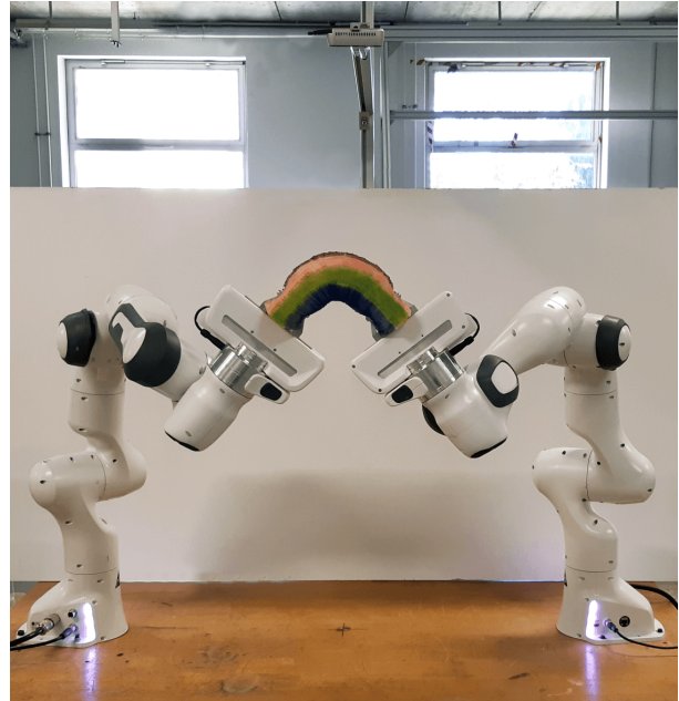
Fig. 1. Our experimental setup with two Franka Emika robots manipulating a foam octagonal cylinder. An overhead 3D camera provides the input for our approach.
