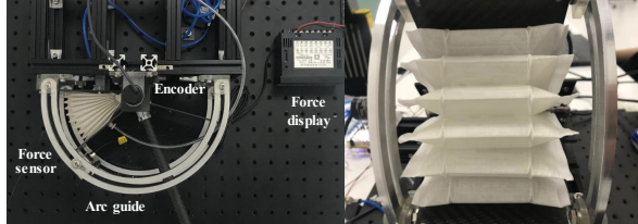
Fig. 8. Experimental setup for testing output torque.
