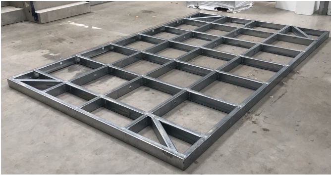
Fig. 2: Light steel-rolled beams automatically cut and punched to size, and manually assembled and fastened. Such assemblies take a lot of time and effort as each beam and assembly can be unique within a prefabricated building.
